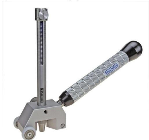
The well proven ERICHSEN Hardness Test Pencil 318 has been improved decisively years ago in the form of a parallel design, Mod. 318 S, with rolling test head.
