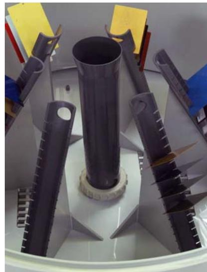
**Specimen holders for weathering panels**
