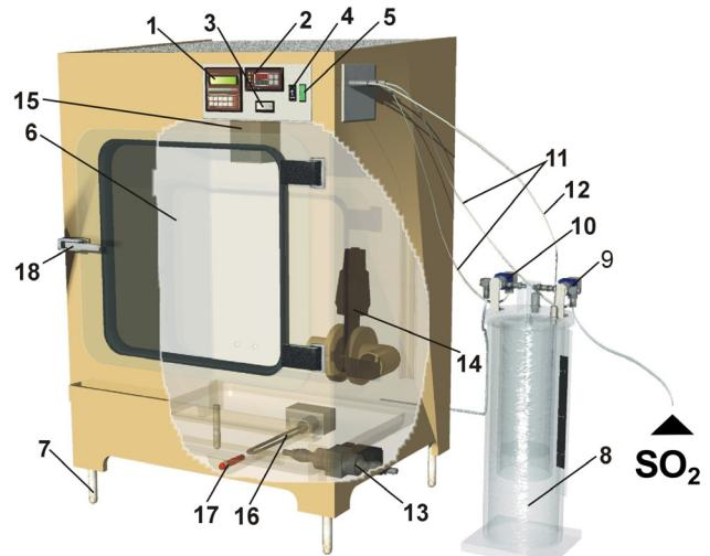
This automatic version also includes a gas injector for tests in SO<sub>2</sub> containing atmosphere.
