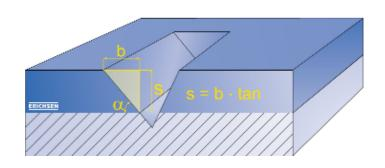
For adhesion tests in accordance with AS 1580 Meth. 408.1, the width of the area where the coating has flaked off during the cutting operation is related to proiection b.
