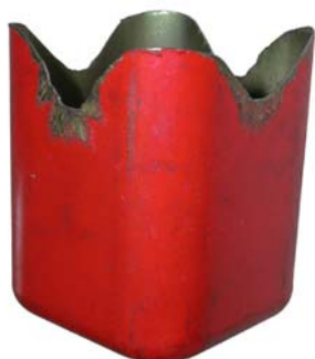
Square Deep Drawing Cup Test
