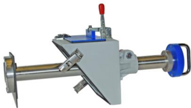
Attachment for tests in accordance with Daimler DBL 5416 (for Mod. 508 VDA)
