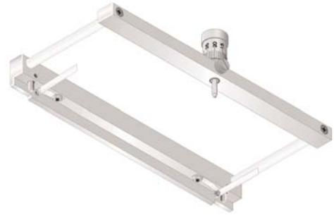
Fig. 6 Film Applicator MULTICATOR 411, with micrometer screw
