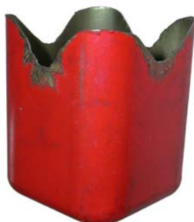
Square Deep Drawing Cup Test
