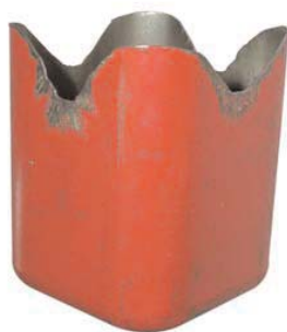
Square Deep Drawing Cup Test
