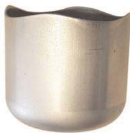
Deep Drawing Cup Test
